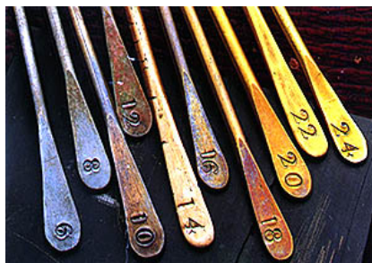
Touchstone set used in the 19th century for testing the fineness of gold
